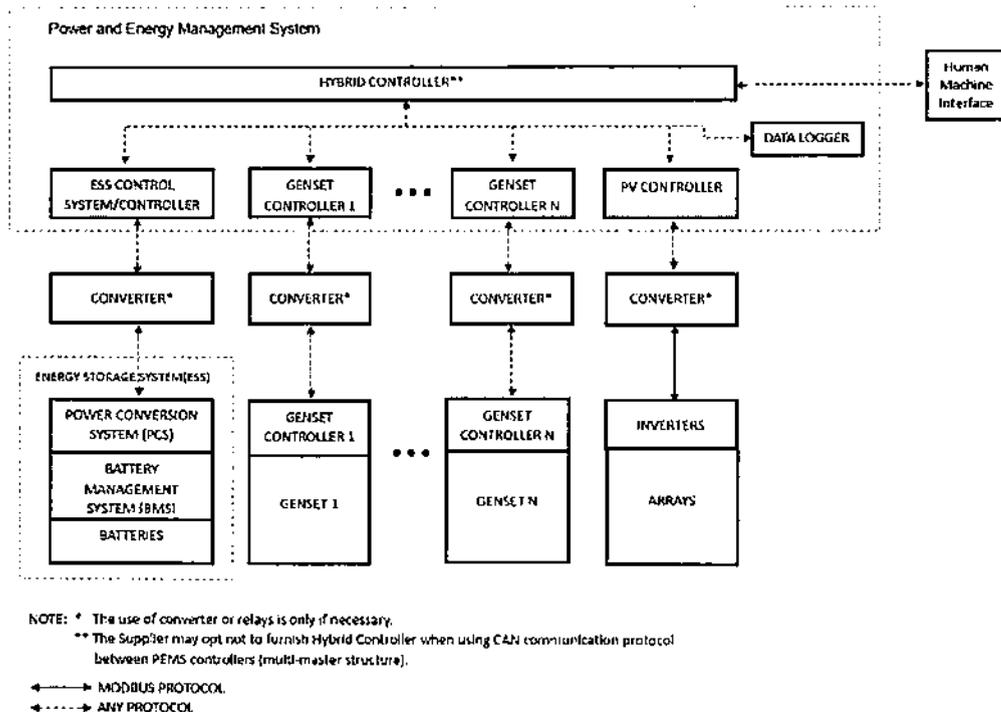
Figure 1: PEMS and Communication Diagram
