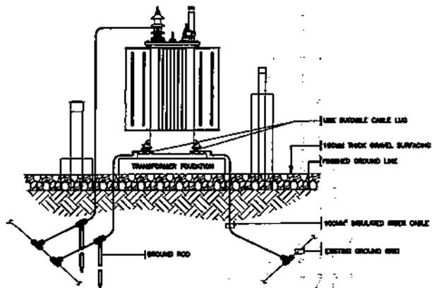
TRANSFORMER GROUNDING CONNECTION (SECTION)
