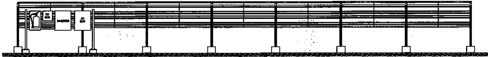
**REAR ELEVATION WITH FIRE EXTINGUISHER, DC BOX, INVERTER & AC BOX**
